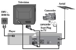
If you have connected your camcorder in this way, you can also connect a scart lead from "AV2" on the back panel of the player to the television. To use this function, see page 15.
